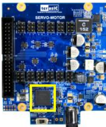
Figure 2-12 CPLD for Power Monitor
